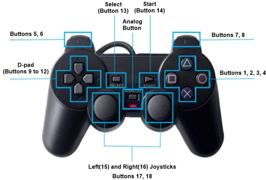
Figure 1: Joystick controls used in this work
